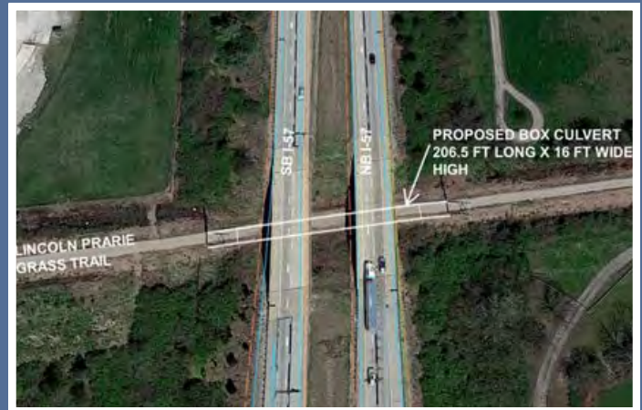
Figure 72. Proposed box culvert replacing bridges over the Lincoln Prairie Grass Trail, IDOT
